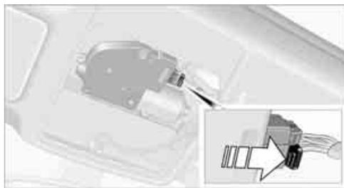
5. Insert the Allen wrench\* supplied with the onboard tool kit, refer to page 223, into the opening provided. Move the glass roof in the desired direction.
