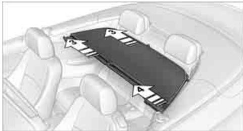
4. Press the wind deflector into the openings, arrows 3, overcoming the tension in the springs, and push the free locking pin in the same direction, arrow 4.
