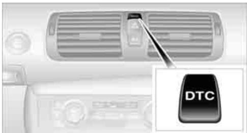
Press the button; the indicator lamps for DTC in the instrument cluster come on.
