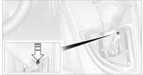
3. Using the screwdriver from the onboard tool kit, refer to page 223, press the red lever, see arrow, while moving the selector lever to the desired position.
