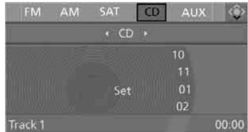
4. If necessary, move the highlight marker to the second field from the top. On cars with a CD changer, select "CD" and press the controller to start the CD player.
