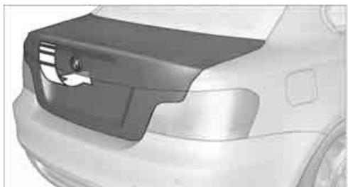
Press the button, see arrow, or the
