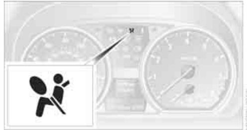
As of radio readiness, refer to page 58, the warning lamp comes on briefly to indicate that the entire airbag system and the belt tensioners are operational.
