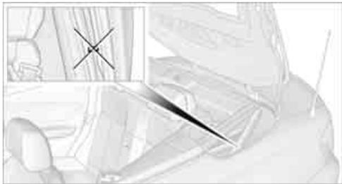
5. Lift out the front part of the convertible top, arrows **4**, on both sides and swing it forward. At the same time keep the convertible top box cover from closing, e.g. using your shoulder.
