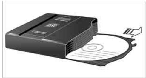
When loading CDs into or removing them from the CD magazine, hold them at their edges and do not touch the reflective signal-sensing area.
