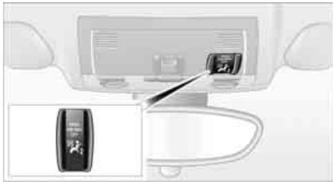
The indicator lamp for the front passenger airbags shows the functional status of the front passenger's front and side airbags in accordance with whether and how the front passenger seat is occupied. The indicator lamp shows whether the front passenger airbags are activated or deactivated.
