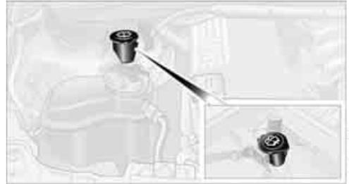
All washer nozzles are supplied with washer fluid by the same reservoir.
