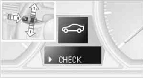
1. Push button **1** in the turn indicator lever up or down repeatedly until the appropriate symbol appears in the display, accompanied by the words "CHECK".
