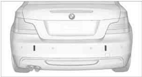
The mounting points are located under the protective covers in the bumper.
