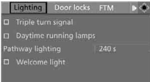
6. Select "Triple turn signal" and press the controller.
