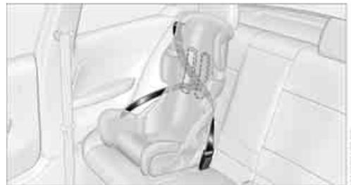
The rear safety belts and the front passenger's safety belt can be prevented from being pulled out in order to fasten child-restraint systems.
