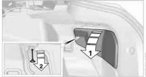
2. Pull the button with the fuel pump symbol down.
