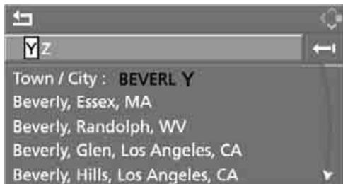
5. If necessary, move the highlight marker to the third field from the top. Turn the controller until the city or town name is selected from the list and press the controller.
