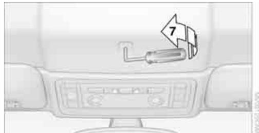
10. Turn the Allen wrench all the way to the left, arrow **7**, until the front convertible top frame is locked to the windshield frame. The rear convertible top frame is automatically pressed down onto the convertible top box cover and is sealed tight under tension.
