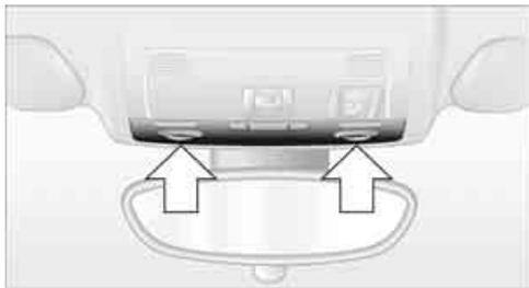
2. On both sides, use the screwdriver to press on the clip inside the opening.
