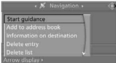
After the route has been calculated, destination guidance is indicated by arrows or a map display on the Control Display.
