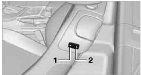
To move the front seats forward or backward from outside or from one of the rear seats: with the door open, press the front end **1** or rear end **2** of the switch.
