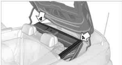
6. Position the rear convertible top frame upright, arrow **5**, and close the convertible top box cover, arrow **6**. Then lower the rear convertible top frame.
