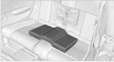
3. In the cargo bay: press the two recesses together and fold down the cover.
