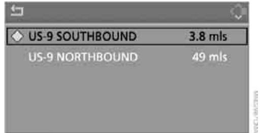
Traffic information on the planned route is shown first, sorted by distance from the vehicle's current position.
