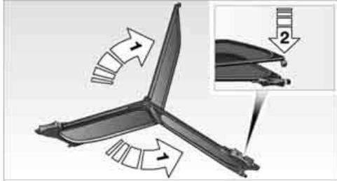
2. Press together the top and bottom parts of the wind deflector until the catch engages, arrow 2.
