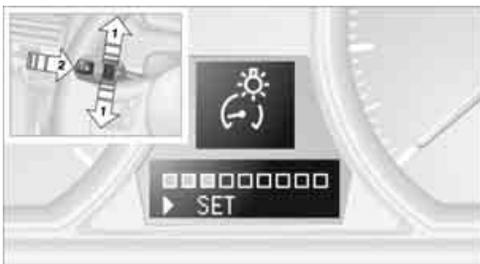
1. Push button **1** in the turn indicator lever up or down repeatedly until the appropriate symbol appears in the display, accompanied by the brightness level and the word "SET".
