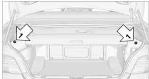
4. Using the screwdriver, loosen the two buttons in the cargo bay, arrows 1, and pull them out forcefully as far as they will go. The convertible top box cover is unlocked.
