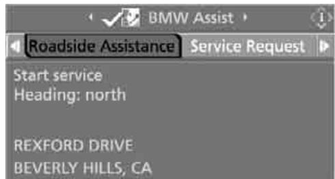
If the current location can be determined, the current vehicle position is displayed.
