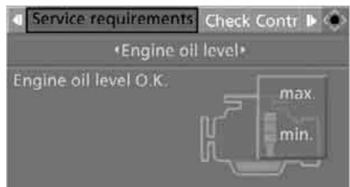
6. If necessary, move the highlight marker to the second field from the top. Turn the controller until "Engine oil level" is selected and press the controller.
