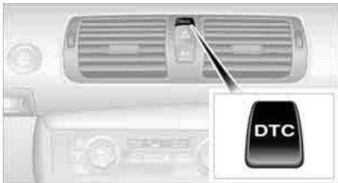
Press the button for at least 3 seconds; the indicator lamps for DSC in the instrument cluster light up. Dynamic Traction Control DTC and DSC have been simultaneously deactivated. Stabilizing and drive-output promoting actions are no longer executed.
