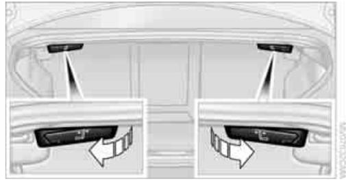
1. To release the rear seat backrest, pull the corresponding lever in the cargo bay.
