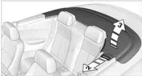
4. The locking pins must have engaged completely. If they are still visible: close the convertible top box cover as far as necessary until the locking bolts engage audibly, then slowly open the cover. During this process, do not close the convertible top box cover completely.
