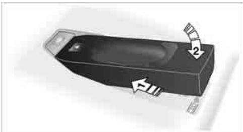
To remove the snap-in adapter:
