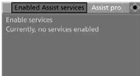
6. Select "Enable services" and press the controller. BMW Assist is activated and data exchange with the BMW Assist Response Center begins.
