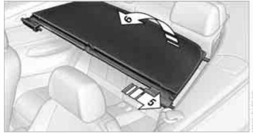
6. Fold up the top section of the wind deflector, arrow 6.
