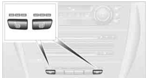
Press once for each temperature level. Three LEDs indicate the highest temperature.
