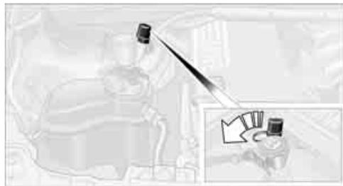
2. Attach one terminal clamp of the plus/+ jumper cable to the positive terminal of the battery or a starting-aid terminal of the vehicle providing assistance.
