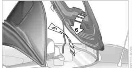
7. Together with another person, press down the front convertible top frame from the outside and on both sides as far as possible.
