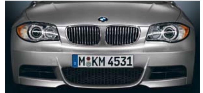
**Front apron** sits below the BMW double kidney-shaped grille with chrome slats. This feature, which brings a constant flow of fresh air to the engine, adds to the front's impressive athletic profile. The central air intake is flanked by two side air intakes that cool the brakes. Two side flaps accentuate the broad front.
