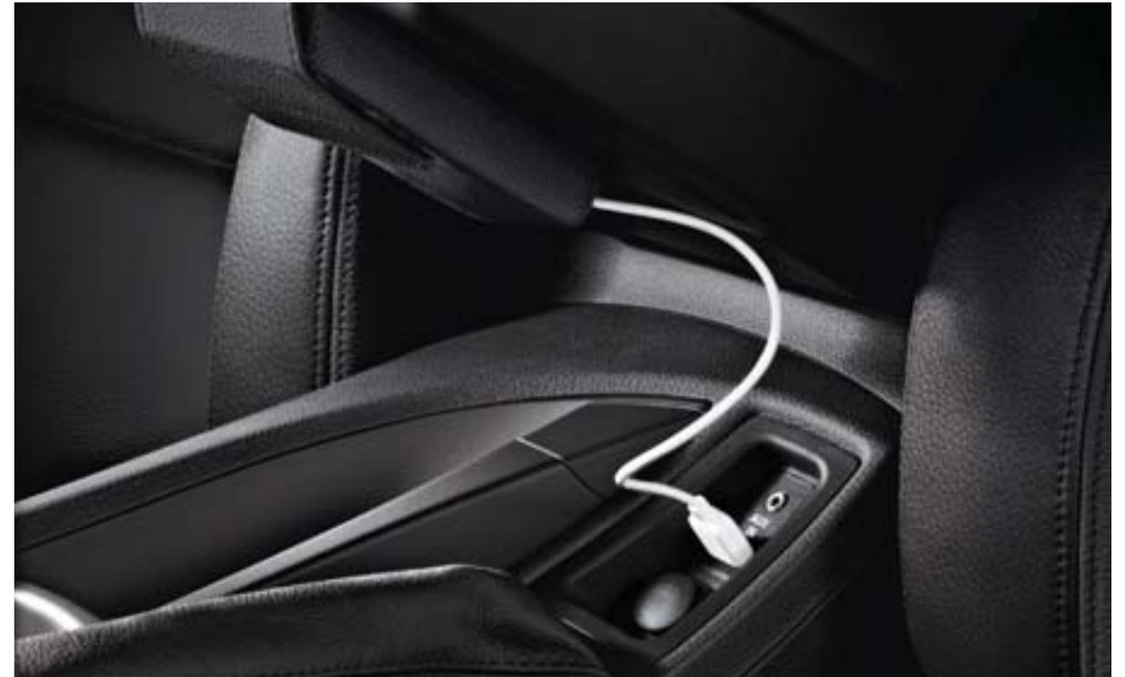
■ **Auxiliary input port** lets you connect an external audio source, such as an iPod® or MP3 player.
