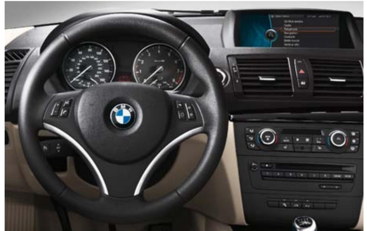
■ **Three-spoke leather-wrapped multi-function steering wheel** lets you keep both hands on the wheel while adjusting various comfort functions, such as controls for audio system and hands-free phone controls (if so equipped).
