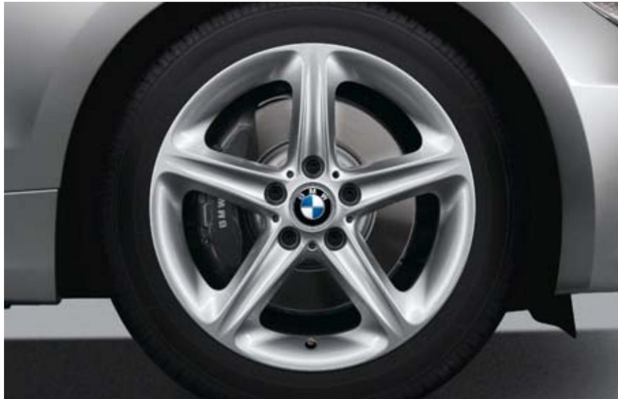
□ **Star Spoke (Style 264) light alloy wheels and run-flat<sup>1</sup> performance tires.**<sup>2</sup> In front: 18 x 7.5 wheels and 215/40 tires; in back: 18 x 8.5 wheels and 245/35 tires.<sup>3</sup> (Included in 135i Sport Package.)
