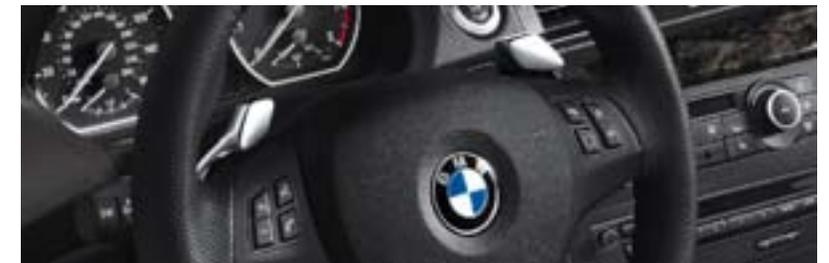
**Steering wheel-mounted paddle shifters**, shown with the three-spoke, leather-wrapped multi-function M sport steering wheel, allow you to shift gears manually without a clutch. This optional feature comes included in the 1 Series Convertible when it is equipped with optional STEPTRONIC automatic transmission and optional Sport Package.
