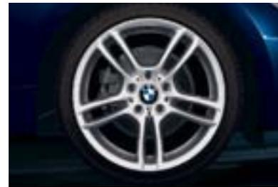
**BMW Double Spoke (Style 261 M) light alloy wheels and run-flat<sup>2</sup> performance tires.<sup>3</sup>** In front: 18 x 7.5 wheels and 215/40 tires; in back: 18 x 8.5 wheels and 245/35 tires. (135i M Sport Package)
