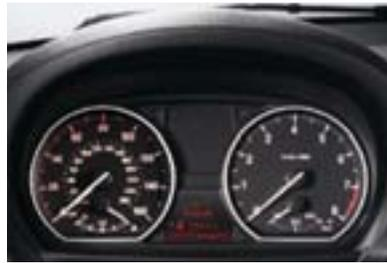
■ **Instrument panel** features a red backlit speedometer and tachometer. Centered between the two easy-to-read analog instruments is the on-board computer (see at right) with liquid crystal display providing additional important driving information.
