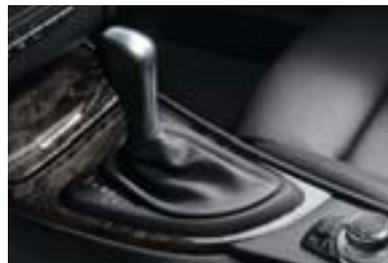
□ **6-speed STEPTRONIC automatic transmission** provides a choice of three modes: Drive, which incorporates BMW's Adaptive Transmission Control; Sport automatic, for a more dynamic shift pattern; and STEPTRONIC automatic, for the hands-on control of a manual without using a clutch.
