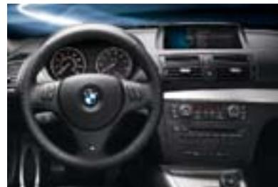
**Three-spoke, leather-wrapped multi-function M sport steering wheel** is included in the M Sport Package. The thick, textured rim and thumb indents are designed for performance driving, while multi-function buttons allow you to adjust various comfort features while keeping both hands on the wheel.
