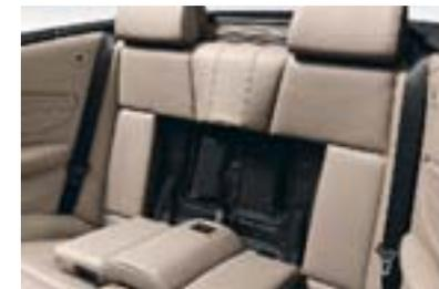
□ **Through-loading hatch** opening includes a **cargo bag** to protect skis, snowboards, and other long items being transported. The cargo bag also serves to protect the interior cabin and trunk surfaces as well. The removable section of the backrest can be laid down and will remain securely in place. (Optional and included in Cold Weather Package.)
