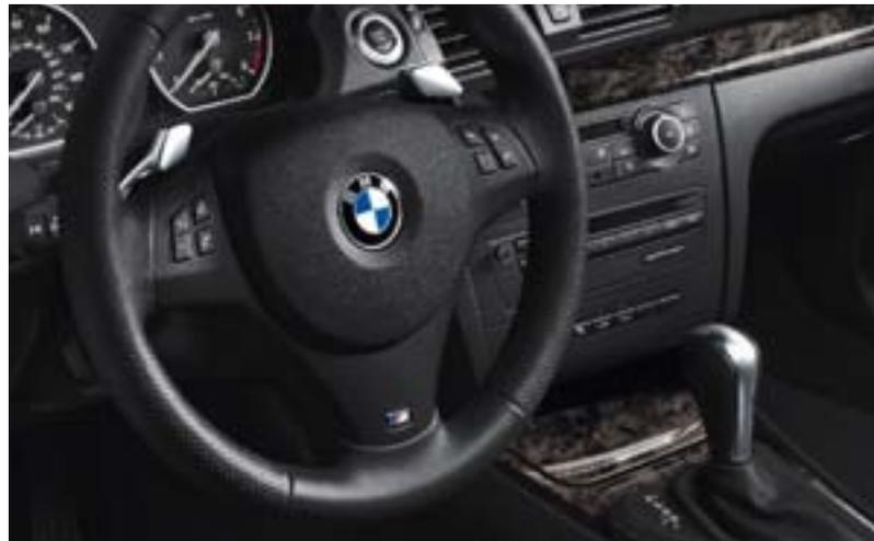
□ **Steering wheel-mounted paddle shifters** allow you to shift gears manually without a clutch. This optional feature comes included in the 1 Series Convertible when it is equipped with STEPTRONIC automatic transmission and M Sport Package or 135i Sport Package.
