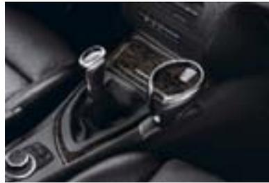
□ **Cupholders** in vehicles with the optional Navigation system are located on the center console and in the passenger footwell. The console-mounted cupholder is detachable for stowing in the glove compartment.
