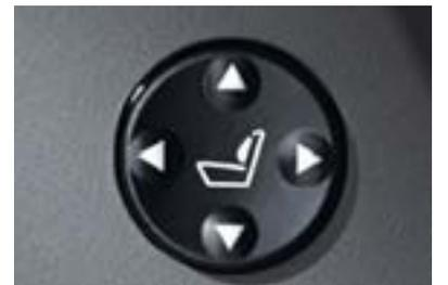
**Lumbar support** for front seats adds four-way power-adjustable comfort for the lower back. Lumbar support can be adjusted up/down and in/out.
