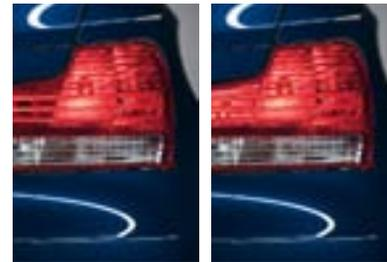
■ **Adaptive Brake Lights** increase vehicle visibility and signal the intensity of your braking action. In the event of an emergency stop, the illuminated area of the brake lights is increased, so traffic following behind you is warned to stop quickly.
