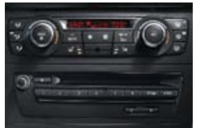
■ **Automatic climate control system** allows occupants to select a specific cabin temperature and choice of fan speeds, as well as automatic or manual airflow and recirculation. Convertible mode also reacts to exterior temperature and sunlight. The automatic recirculation control activates whenever certain air pollutants are detected. The system also includes defrost/demist and MAX A/C functions.
