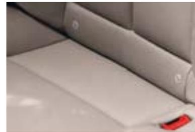
■ **ISOFIX child seat attachment** on the rear seats provides secure, safe attachment of a child seat with clip-in plug connectors, plus additional fastening points on the upper part.
