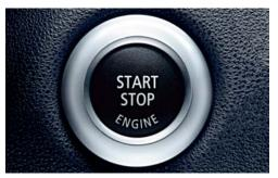
■ Start/Stop button to start and stop the engine, in conjunction with the radio remote control unit.
