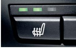
☐ **Seat heating** (with 3 levels) for driver and front passenger, seat surface and backrest can be heated for an almost instant cosy feeling of warmth.
