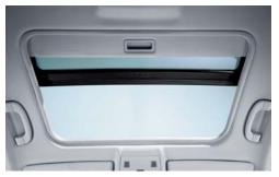
☐ Glass sliding/vent roof, electric, with comfort opening function via the remote control unit.
