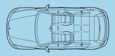
$All \ dimensions in \ millimetres. \ Luggage \ compartment \ capacity \ (measured \ according \ to \ VDA \ standard) \ approx. \ 330 \ to \ 1,150 \ litres \ (11.7 \ to \ 40.6 \ cu \ ft).$
