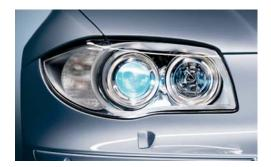
☐ Xenon light for low and high beam, including four parking light rings and dynamic headlight range control, for better road illumination at night or in bad weather.
