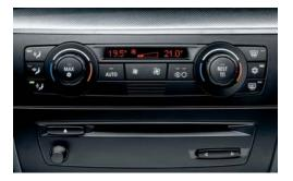
☐ Automatic air conditioning (shown here), with AAR, microfilter, fogging and solar sensors and residual heat button, quickly establishes and maintains the selected temperature. With separate temperature control for left and right sides.
