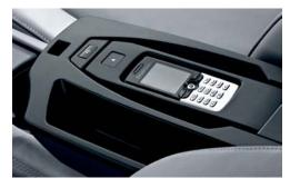
□ Preparation for mobile telephone with Bluetooth interface (with hands-free system, connection for recharging and external aerial). A separately available snap-in adapter enables connection of a Bluetooth-compatible mobile phone, which can also be operated via the iDrive Controller (in conjunction with navigation system). For mobile phone options contact your BMW partner.
